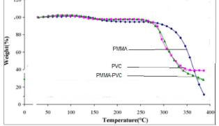
Figure (3.2 a): TGA thermograms of PVC, PMMA and PVC/PMMA.
