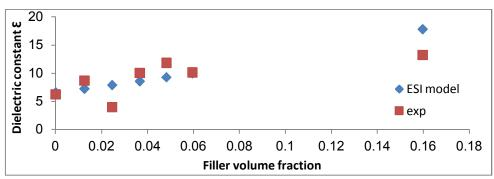
Figure (3.6): Relation between the dielectric constant and the filler volume fraction for all samples.
