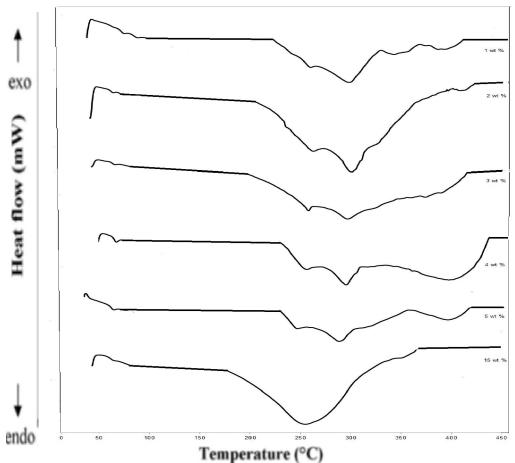
Figure (3.1b): DSC thermograms of all PVC/PMMA loaded conductive polypyrrole composites.
