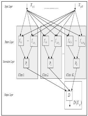
Fig. 1. Structure of the original probabilistic neural network
