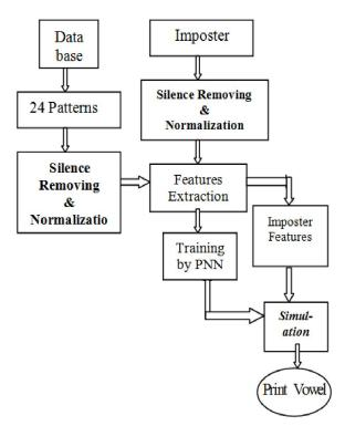
Fig. 2. Flow chart for proposed system
