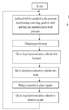
Figure 3. Pressure assembly process action process
