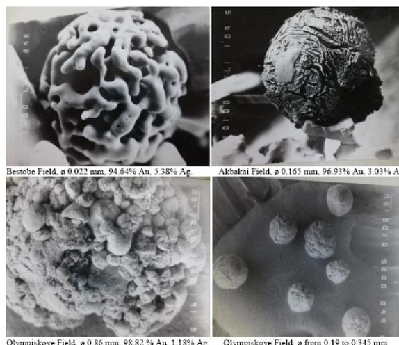
**Fig. 11. Spherical forms of metallized gold clusters.**
