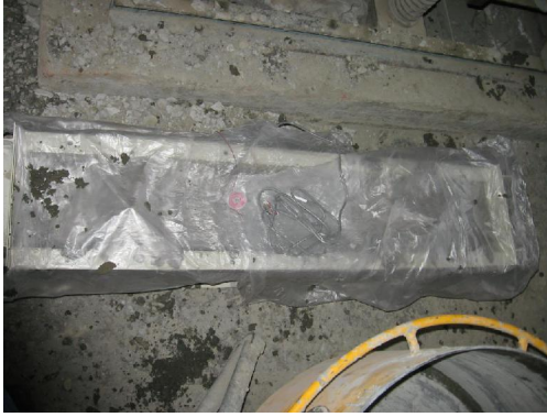
Figure 7. Beam immediately after pouring
