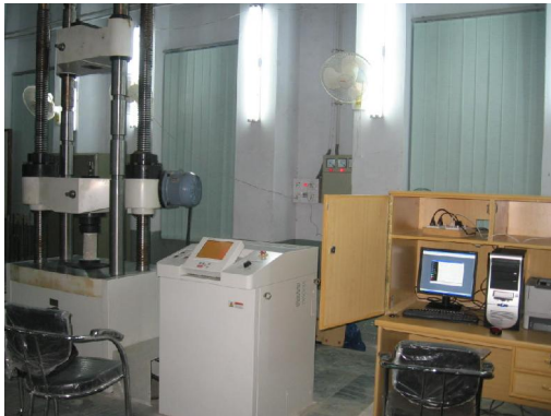
Figure 8. Compressive strength test in UTM
