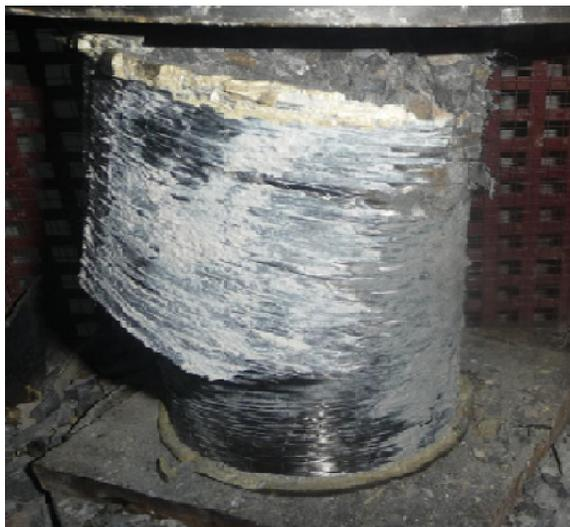
Fig.2 (B) Rupture of cylinder wrapped with FRP
