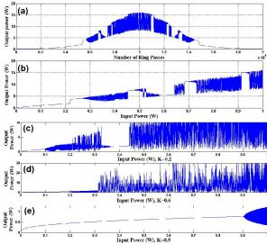
Fig. 2: The chaotic signal generation within the single ring resonator
