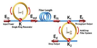
**Fig. 1:** A fiber optic ring resonator is constructed to an add/drop filter system by the couplers
