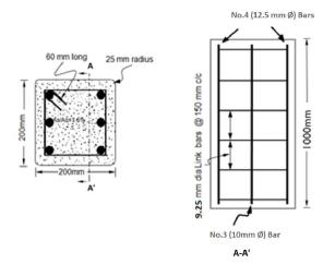
Fig. 1. Steel reinforcement bars arrangement in square concrete columns.
