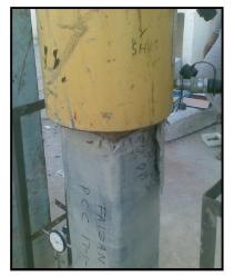
Fig.11 Failure mode of CFRP confined column
