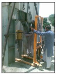
Fig.8 Arrangement of concrete column in axial load test up
