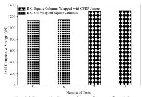
Fig.14 Strength Comparison of unconfined & confined R.C columns
