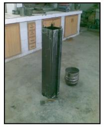
Fig.2 Steel mould for casting of concrete columns
