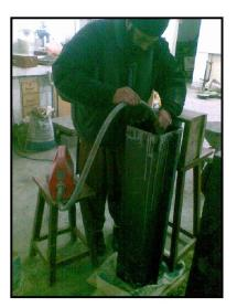
Fig.3 Application of vibration to concrete through internal poker vibrator
