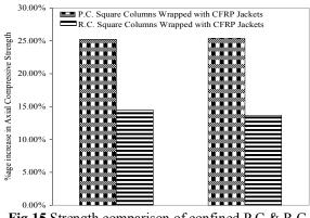
Fig.15 Strength comparison of confined P.C & R.C columns
