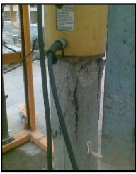
Fig.10 Failure mode of un-confined concrete column
