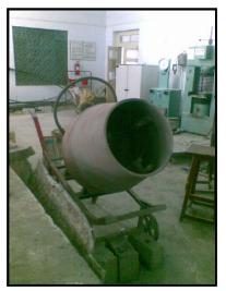
**Fig.4** Concrete mixer for preparation of specimens
