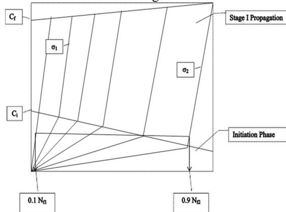
Figure 4. Schematic of initiation & stage I propagation phase
