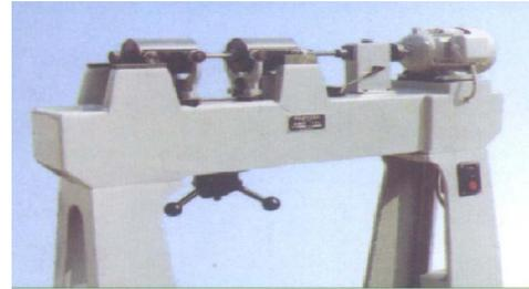
Figure 2 (Rotary bending fatigue testing)
