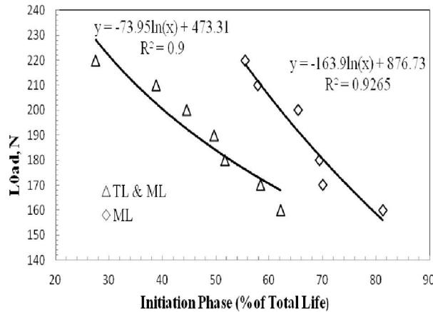
Figure 5 (Crack initiation life in varying amplitude loading)
