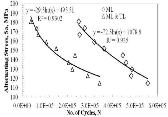
Figure3 (S-N Curves of constant amplitude)
