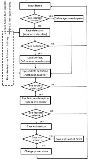
Figure 7. Eye Gaze Tracking Algorithm.
