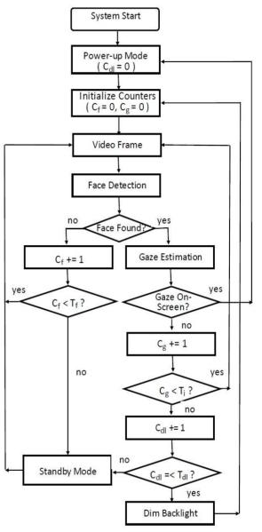
Figure 2. Flowchart of the proposed eye-gaze driven display power management and Conservation system.
