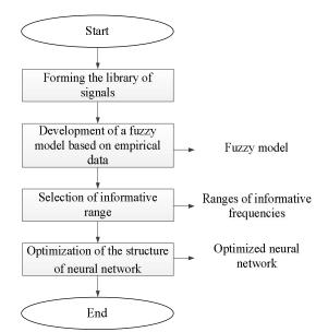
Fig. 4 The algorithm for preparing the ddiagnostic system on a two-step algorithm.
