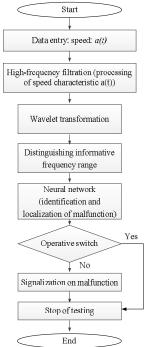
Fig. 1 – Algorithm of NN diagnostics using wavelet analysis and neural network.
