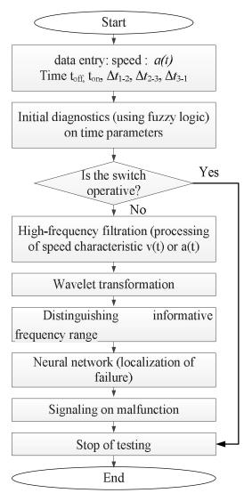
Fig. 3 A two-step algorithm of NN diagnostics using fuzzy model and neural network.
