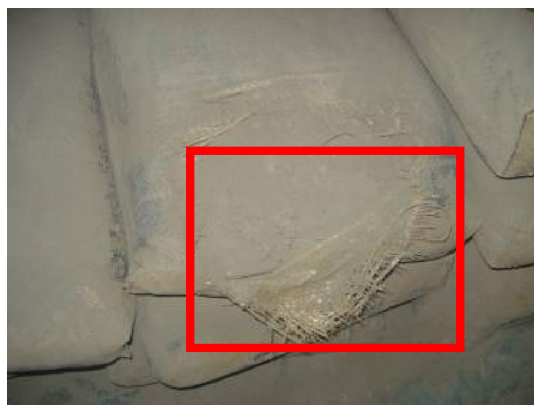
Figure 7: Poor storage of cement bags
