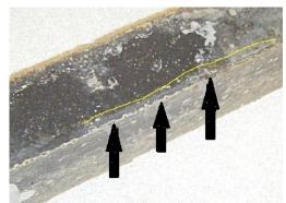
Figure.2: White filled crack in SR Specimen
