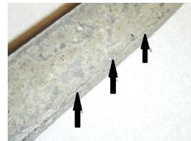
Figure5: Longitudinal crack in ME specimen
