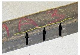
Figure 3: White filled crack in MA Specimen
