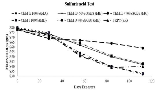
Figure 7: Mass loss of samples after sulfuric acid exposure
