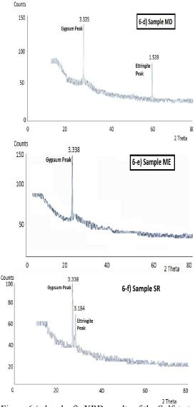
Figure 6 (a,b,c,d,e,f): XRD results of the Sulfate test showing the ettringite and gypsum formation
