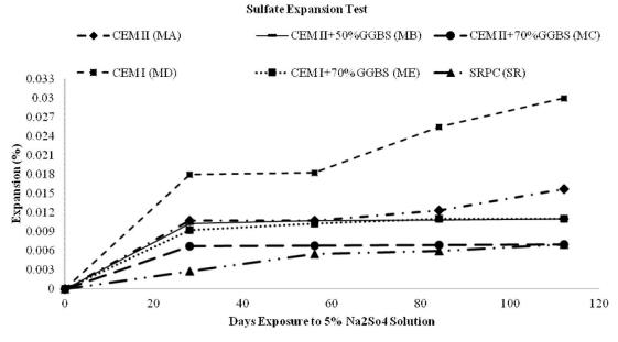
Figure 1: Results of sulfate expansion test
