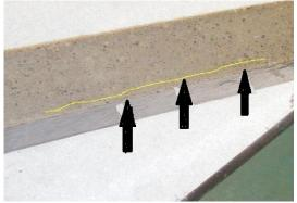
Figure 4: Longitudinal crack in ME specimen
