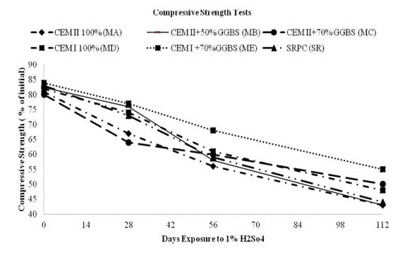
Figure 8: Influence of period of acid exposure on compressive strength
