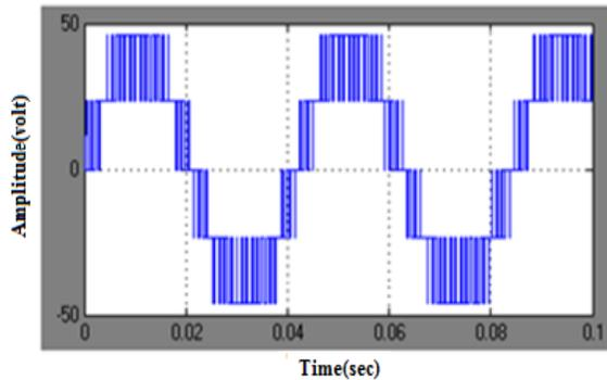
Figure 14. Output voltage waveform for fault free condition
