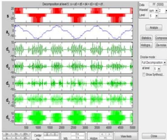
Figure 17. Wavelet transform for fault free FF
