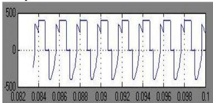
Figure 4. Output voltage waveform for phase A for fault OF4
