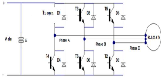
Figure 2. Open Circuit Fault-IGBT1 is assumed to be open
