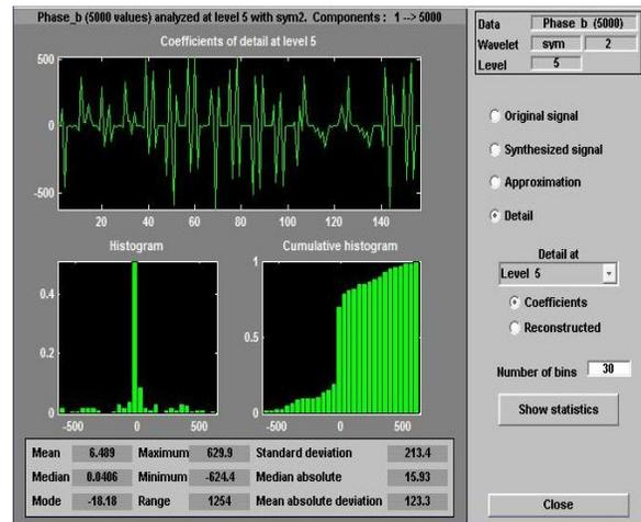
Figure 11. Statistical analysis of wavelet transform for phase B for fault OF4
