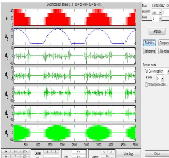
Figure 19. Wavelet transform for Double fault Sa+ and Sa-
