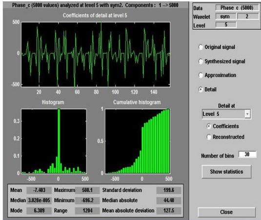
Figure 12. Statistical analysis of wavelet transform for phase C for fault OF4
