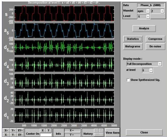
Figure 8. Wavelet transform for phase B for fault OF4
