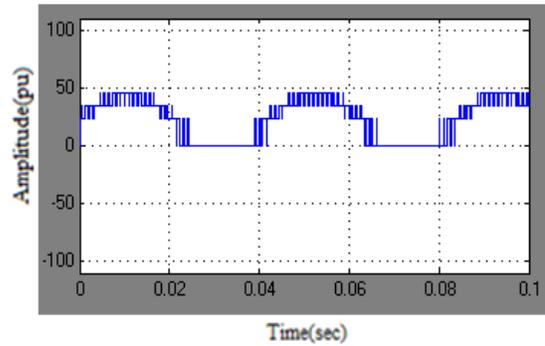
Figure 16. Output voltage waveform for fault Sa+ and Sa-
