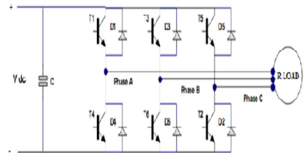
Figure 1. Three phase single level VSI
