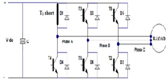
Figure 3. Short Circuit Fault- IGBT1 is assumed to be short circuited
