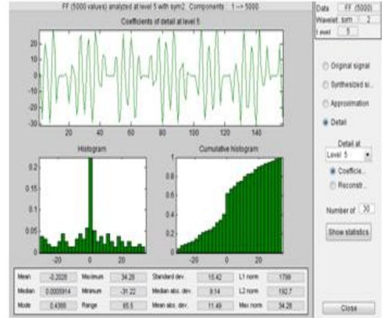
Figure 20. Statistical analysis of wavelet transform for fault free FF
