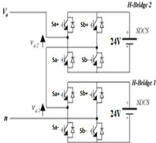
Figure 13. Single phase multilevel inverter
