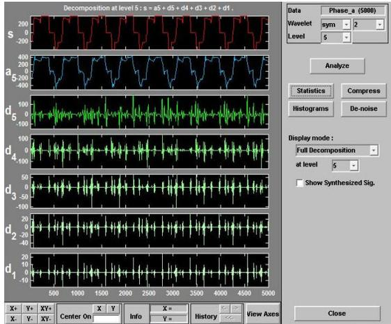
Figure7. Wavelet transform for phase A for fault OF4
