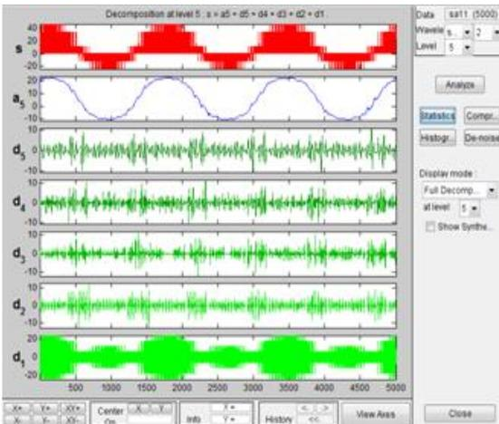
Figure 18. Wavelet transform for single fault Sa+
