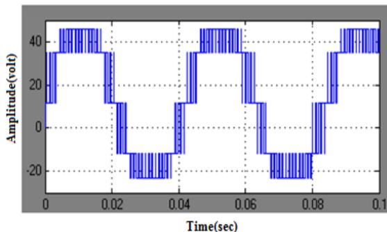
Figure 15. Output voltage waveform for fault Sa+
