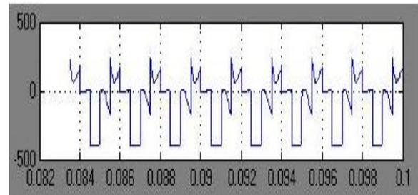
Figure 6. Output voltage waveform for phase C for fault OF4
