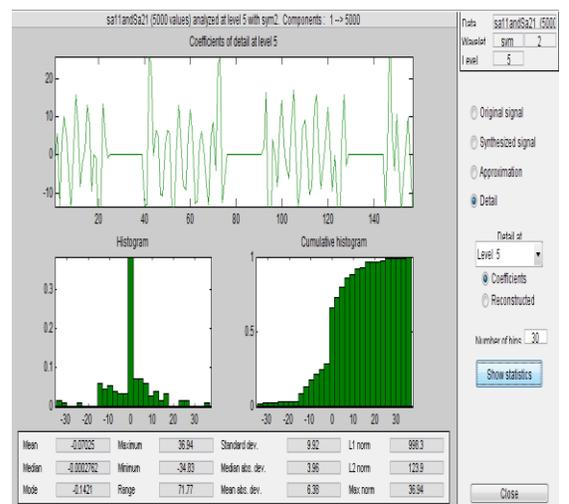
Figure 22. Statistical analysis of wavelet transform for Double fault Sa+ and Sa-
