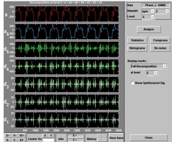
Figure9. Wavelet transform for phase C for fault OF4
