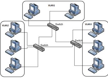
Figure 1. A switched network topology using VLANs.
