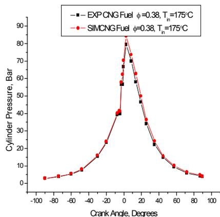
Figure 2. Peak Cylinder Pressure with respect to crank angle at equivalent ratio of 0.38 and inlet temperature of  $175^{\circ}\text{C}$  in both experimental and simulation study
