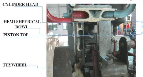
**Figure 1 Engine Model**
