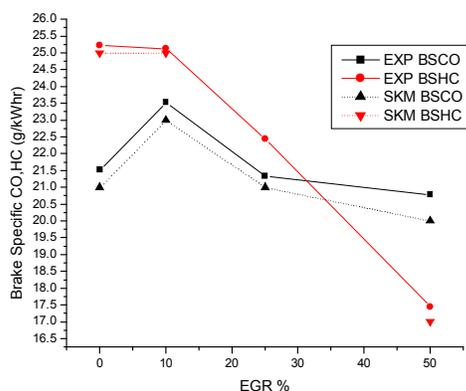
Figure 3. BSCO & BSHC versus EGR at three load condition in both experimental and simulation study.
