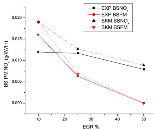
Figure 4. BSPM & BS $\text{NO}_x$  versus EGR at three load condition in both experimental and simulation study.
