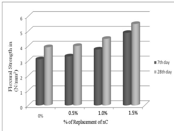
Chart-3: Flexural Strength of Concrete with and without nC (0 – 1.5 %)
