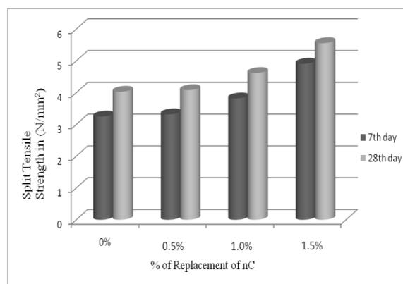
Chart-2: Split tensile strength of Concrete with and without nC (0 - 1.5 %)
