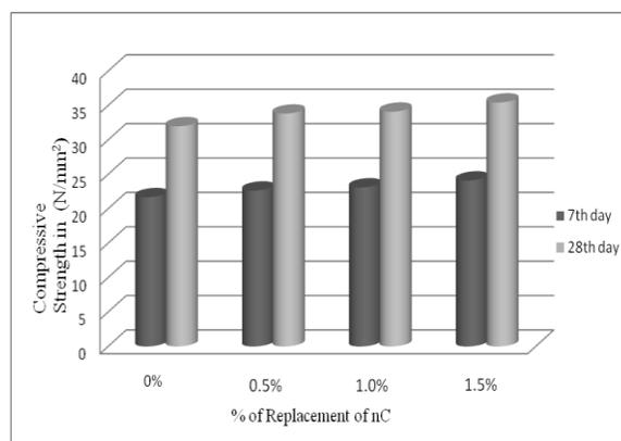
Chart-1: Compressive strength of Concrete with and without nC (0 - 1.5 %)
