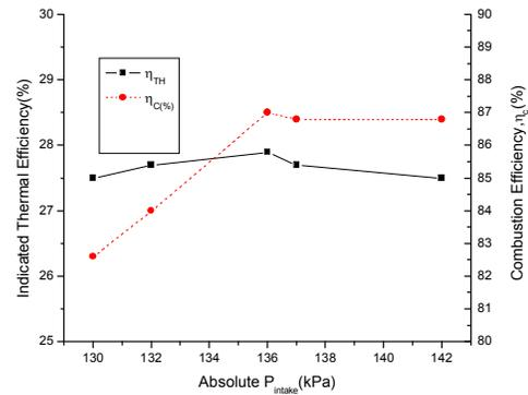
Figure 5. Intake Pressure effect on indicated thermal efficiency and combustion efficiency, CNG HCCI engine
