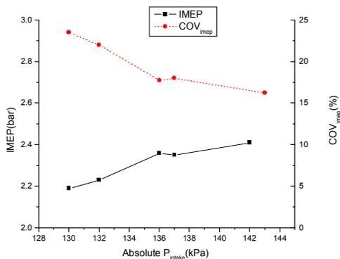
Figure 4. Intake Pressure effect on IMEP and COV<sub>imep</sub> of HCCI engine
