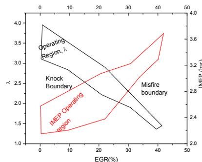
Figure 2. Operating region of CNG HCCI engine with boosted intake pressure and partial fuel reforming
