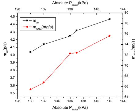
Figure 3. CNG flow rate adjustment with intake pressure to keep constant  $\lambda = 3.62$
