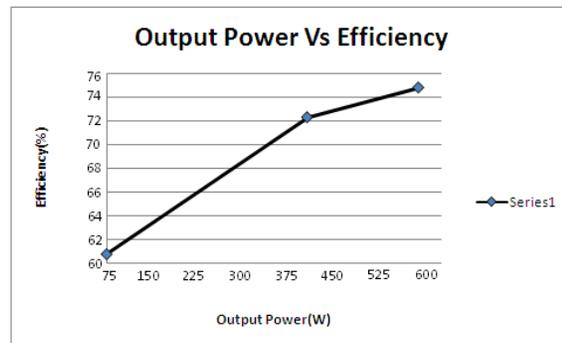
**Figure 8 Output Power Vs Efficiency of FSTPI Fed Induction Motor with Boost Converter**
