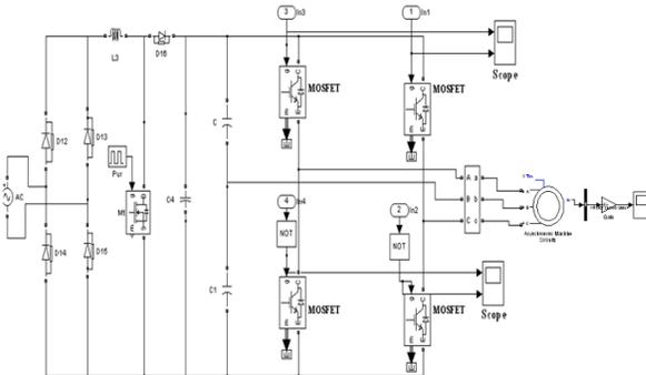
**Figure 3 Four Switch Three Phase Inverter Fed Induction Motor System with Boost Converter**
