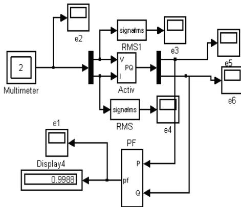
**Figure 4 Power Factor Measurement of Boost PFC Converter**
