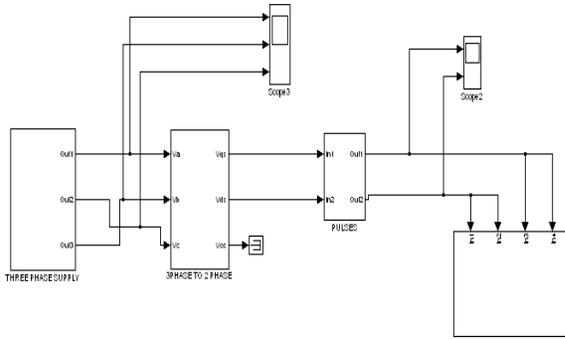
**Figure 2 Simulation Block Diagram of FSTPI Fed Induction Motor Drive System with Boost Converter**
