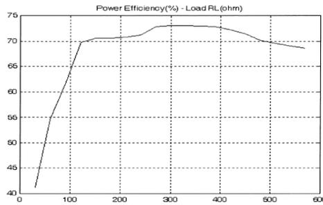
**Figure 9 Output Power Vs Efficiency of CMOS-TG QSC boost DC-AC inverter**
