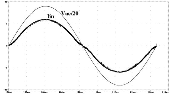
**Figure 5 Power Factor Measurement of CMOS-TG QSC boost DC-AC inverter**
