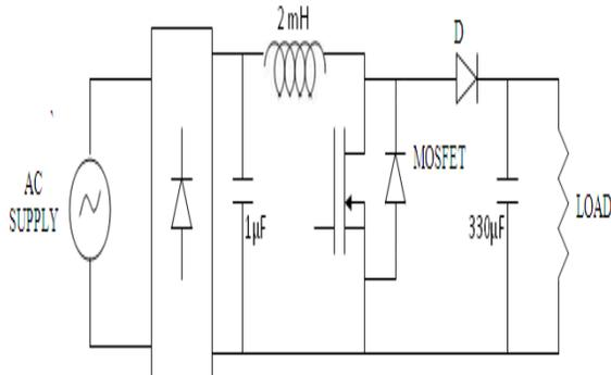
**Figure 1 Basic Boost Converter Circuit**
