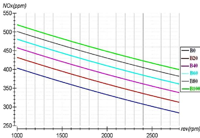
Fig 7. Effect of biodiesel and engine speed on NO<sub>x</sub> emissions at 75% engine load
