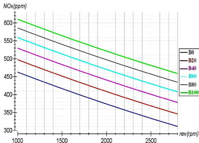
Fig 8. Effect of biodiesel and engine speed on NO<sub>x</sub> emissions at 100% engine load
