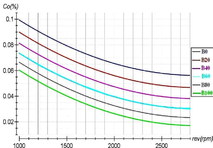
Fig 2. Effect of biodiesel and engine speed on CO emissions at 50% engine load
