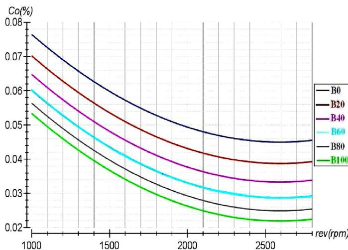
Fig 4. Effect of biodiesel and engine speed on CO emissions at 100% engine load
