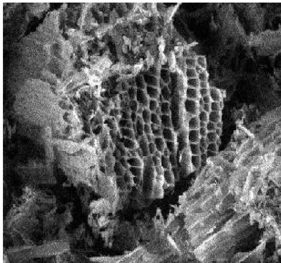
Figure 1: SEM image of activated carbon. A porous structure is observed [16].
