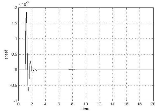
Figure (11) Relation between  $\Delta\omega$  and the time with TCSC
