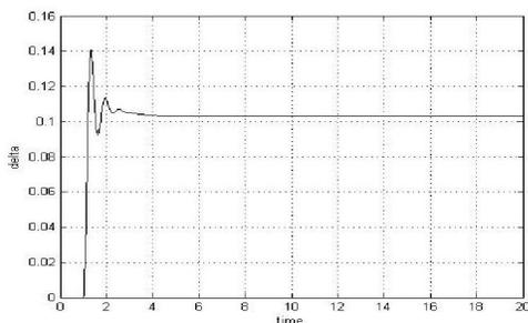
Figure (10) Relation between  $\Delta\delta$  and the time with TCSC
