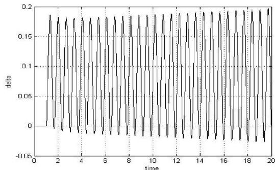
Figure (7) Relation between  $\Delta\delta$  and the time without TCSC device
