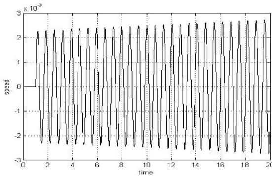
Figure (8) Relation between  $\Delta\omega$  and the time without TCSC
