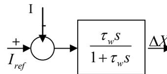
Figure (4) Wash out Circuit of TCSC
