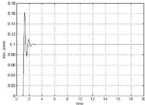
Figure (9) Relation between  $\Delta P_e$  and the time with TCSC
