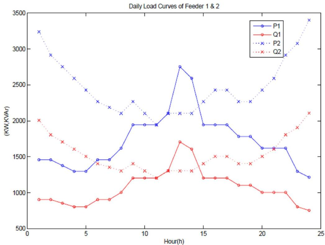
Figure 8: Active and reactive power loading of feeder1 and feeder2
