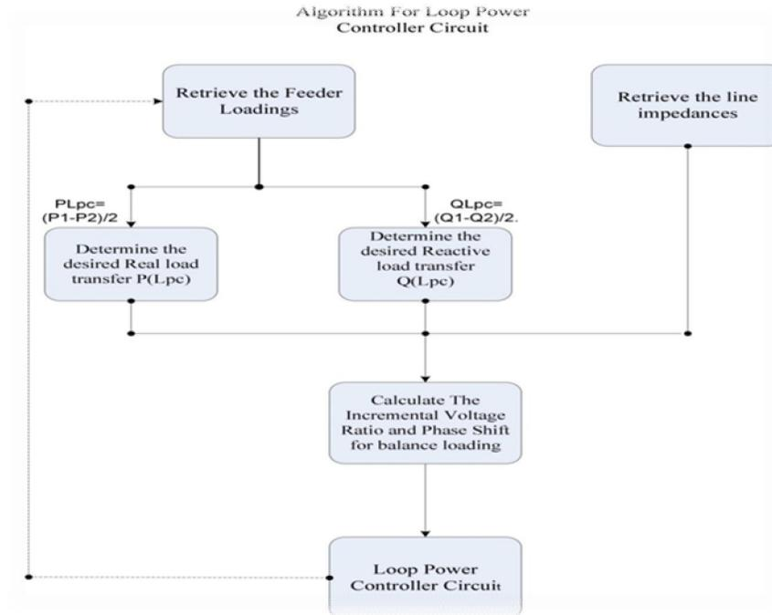
Figure 6: Algorithm Flow Chart of Loop Power Controller (LPC)
