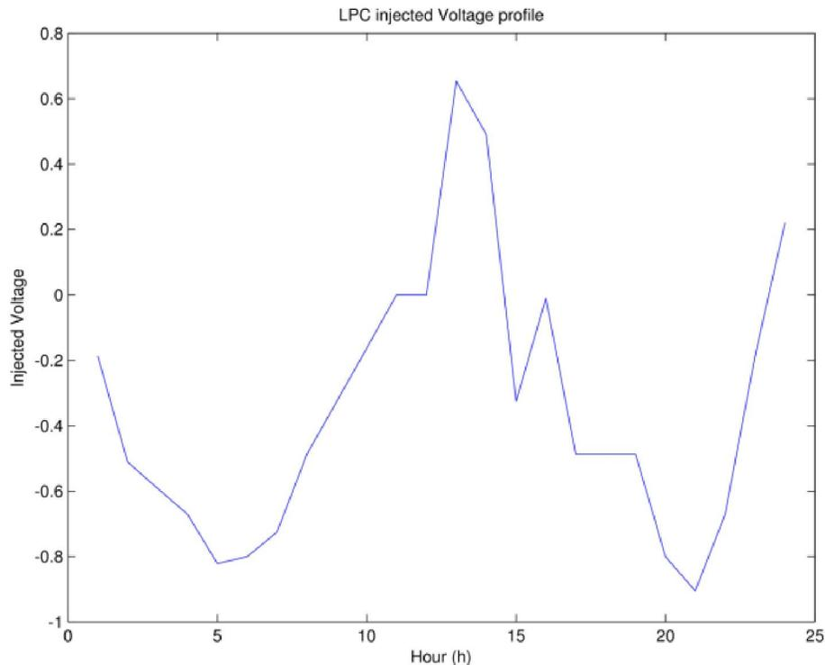
Figure 14: Injected Voltage (P.U) by LPC
