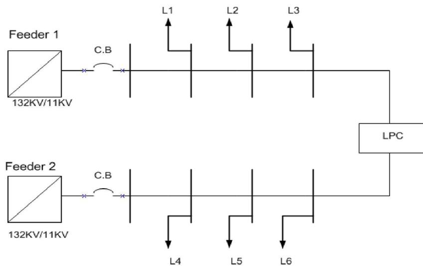
Figure 10: Schematic One line Diagram Distribution feeders with LPC
