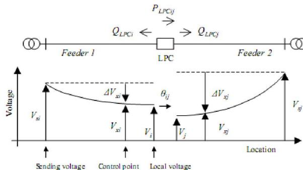
Figure 3: Control Parameters of Loop Power Controller (LPC) [11]
