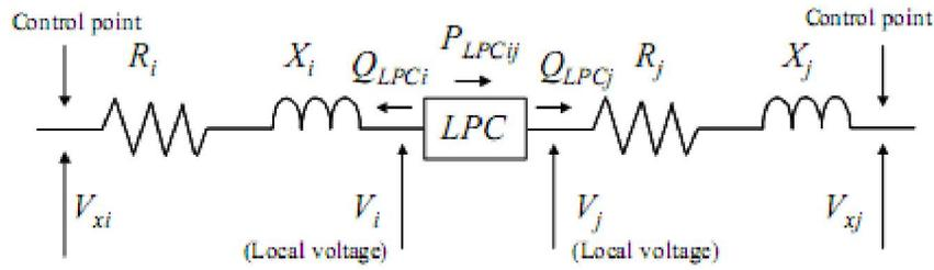
Figure 4: Equivalent Circuit of Loop Power Controller (LPC)
