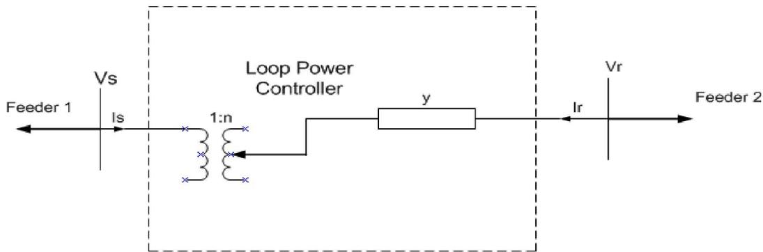
Figure 5: Circuit Model for LPC
