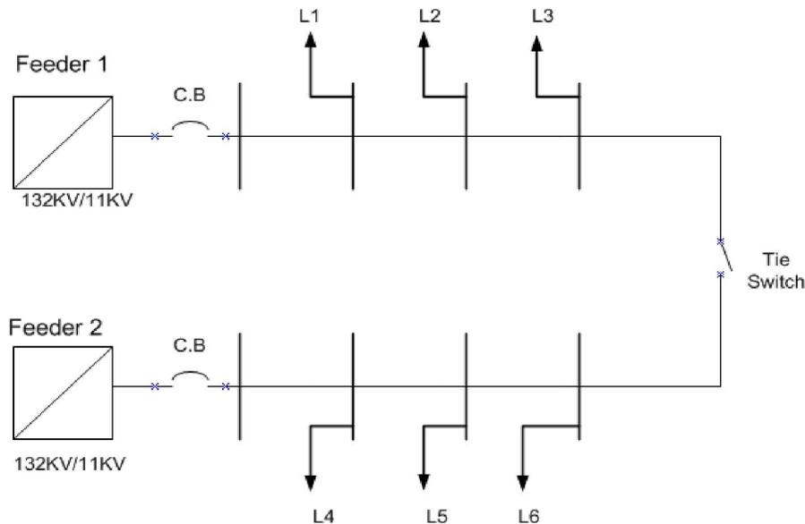
Figure 7: Schematic One line Diagram of Distribution Feeders
