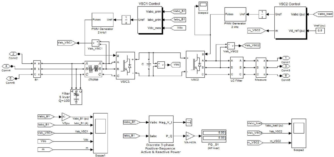
Figure 12: Simulation Diagram of Loop Power Controller
