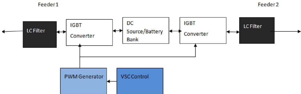
Figure 9: Block Diagram of Loop Power Controller
