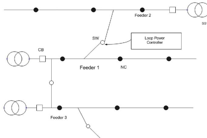
Figure 2: Radial distribution network with loop power controller (LPC)
