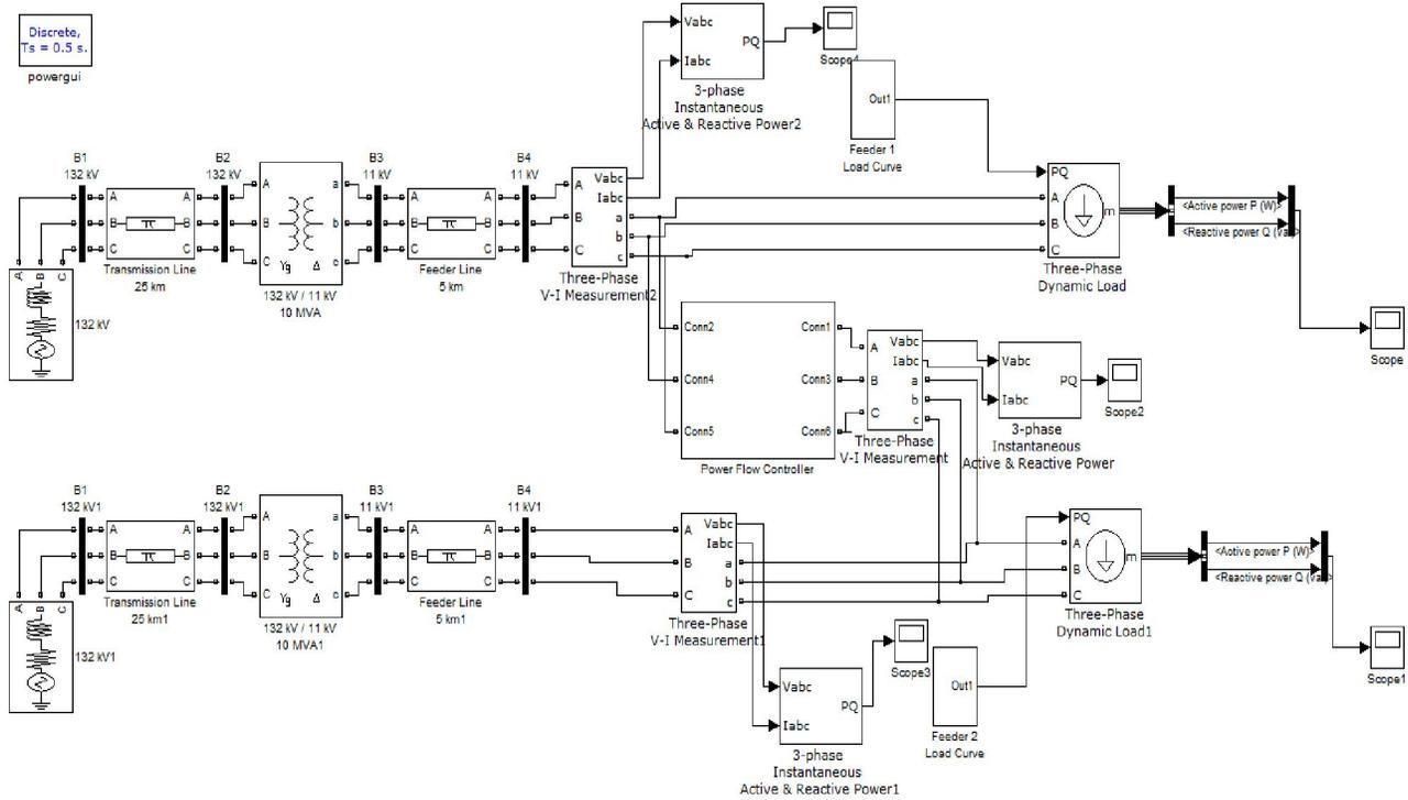
Figure 11: Simulation Circuit of Distribution Feeders
