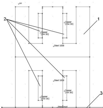
**Figure 4 – 2D-model of magnetic system: 1 - magnetic conductor, magnetizing coils, 3 - tested item.**
