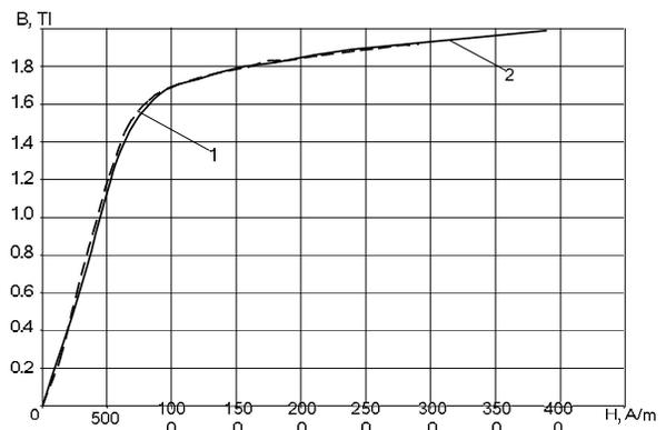
**Figure 8 - Measured magnetization curves: 1 - obtained by means of proposed IMS, 2 - of a sample.**
