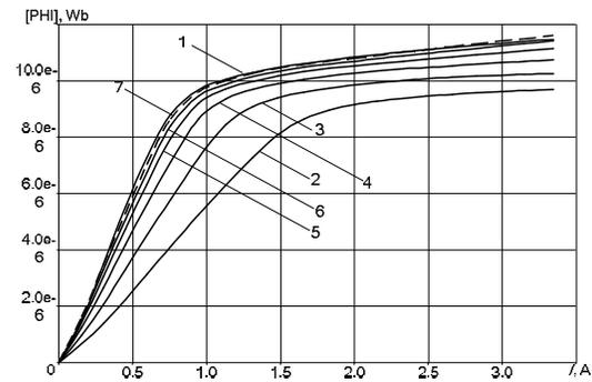
**Figure 7. - Stage-by-stage approximation of dependency  $[PHI]_{ta\_max}(i_{max})$  (curves 2-7), obtained by means of the simulation (model), to experimental characteristic  $[PHI]_{ta\_max ex}(i_{max ex})$  (curve 1)**
