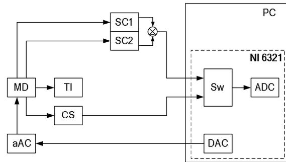
**Figure 2 - Structural diagram of information and measurement system for identification of magnetization curve of sheet electrical steel.**
