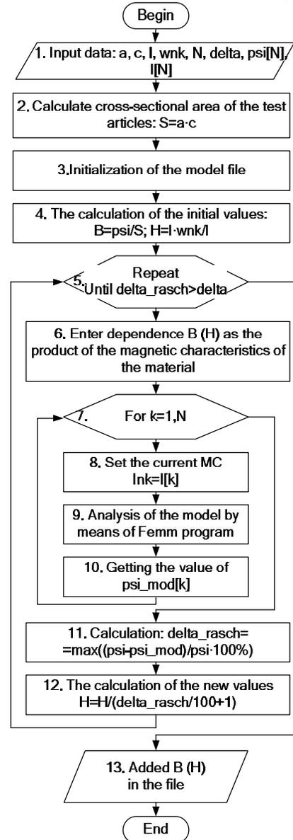
**Figure 5 - Algorithm of recovering of magnetic characteristic of the item's material in accordance with method of experimental and simulation method.**
