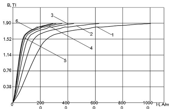
**Figure 6. - Changing of magnetization curve of sample's material  $B(H)$  in order to provide in the model dependency of  $[PHI]_{ta\_max}(i_{max})$  corresponding to the experimental  $[PHI]_{ta\_max ex}(i_{max ex})$ : 1,2,3,4,5 - curves in the process of approximation, 6- resulting (or 'recovered') characteristic of the material.**
