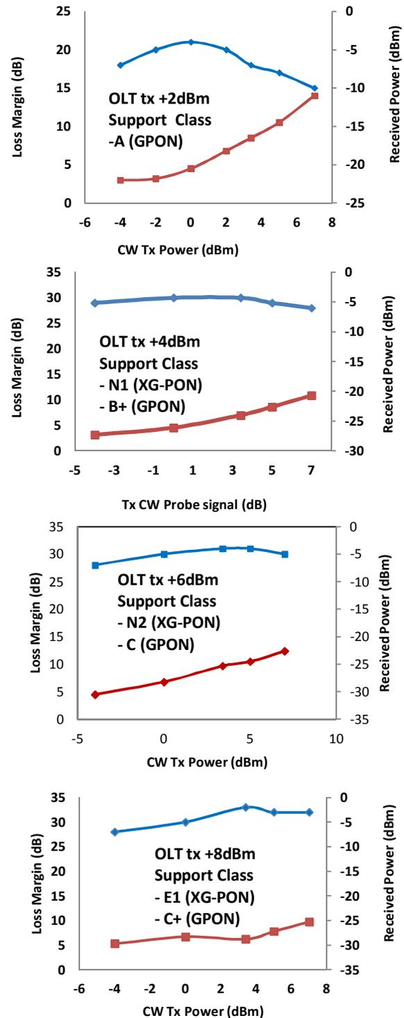
Figure 9: Summary BER $10^{-9}$  line at the 2.5 Gbps OLT downstream transmit signal using the SAC20b transmit power supporting different classes of ODN PON systems
