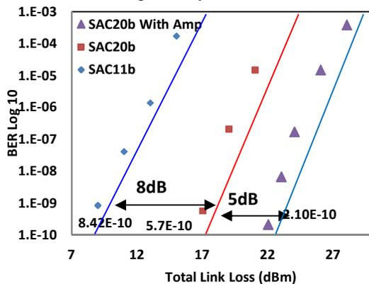
Figure 6: Performance of the system at 2.5 Gbps with and without the post amplifier at the OLT AOPR module
