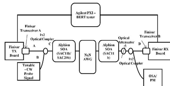
Fig. 3: Experimental setup of the TWDM AOPS PON system configuration
