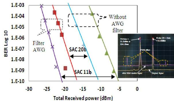
Figure 5: Comparison between the total received power using a booster SOA and an inline SOA before and after AWG filtering at 2.5 Gbps in XGM
