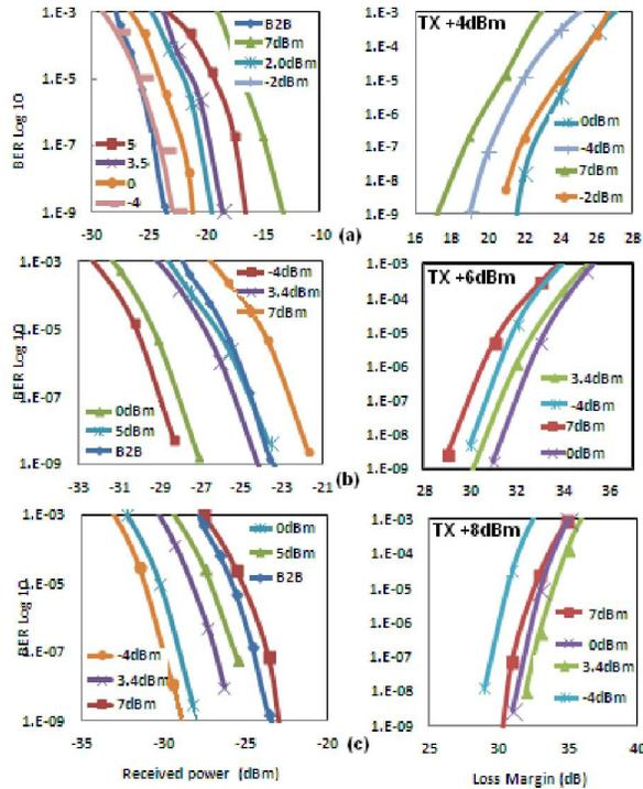
Figure 8: BER line of the 2.5 Gbps OLT downstream transmits a signal using SAC20b with a transmit power of +4, +6, and +8 dBm: (a) ONU average received power and (b) total link loss margin
