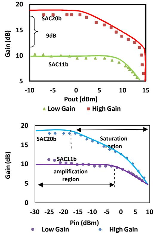
Figure 4: SOA SAC20b and SAC11b gain profiles versus input/output
