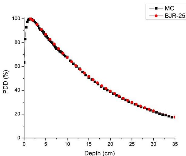
Figure 2: The PDD curves of the conventional 6 MV Varian linac beam simulated (squares) and obtained from BJR-supplement-25 (circles) for a  $10 \times 10 \text{ cm}^2$  field-size in a water phantom.
