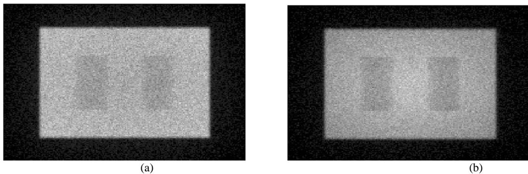
Figure 5: The acquired images of two cylindrical bones with 2 cm diameter placed inside water phantom with 5 cm thickness at 100 cm from the target by (a) the conventional beam and (b) the copper target beam.
