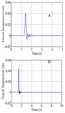
Figure 10: Relative displacement. (A) Active (B) Passive
