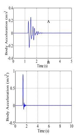
Figure 8- The acceleration on car body. (A) Active (B) Passive
