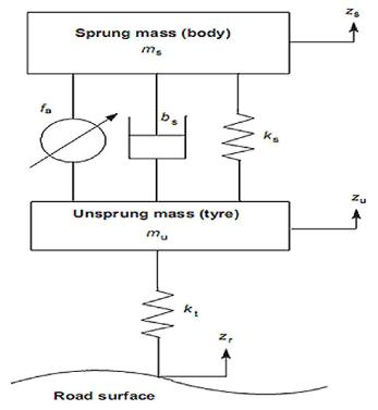
Figure 1: An active suspension system model
