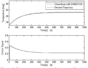
Figure-5 Temperature response for system-II using DSMCFOS (a) Closed loop temperature trajectory and desired trajectory (b) control effort
