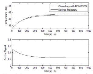
Figure-4 Temperature response for system-I using DSMCFOS (a) Closed loop temperature trajectory and desired trajectory (b) control effort
