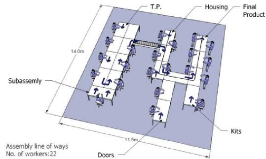
Fig (7) Assembly line for way-type products
