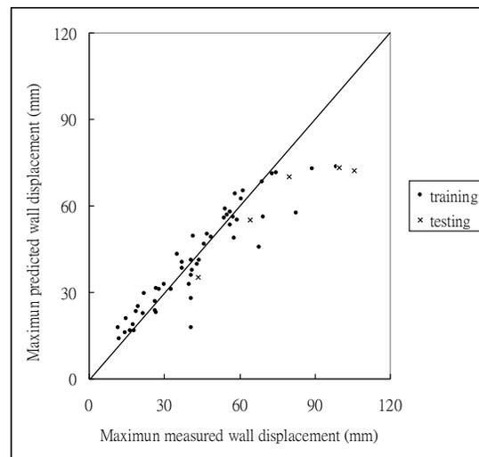
Figure 4. Measured vs. Predicted Maximum Diaphragm Wall Displacements
