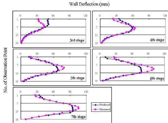
Figure 5. Wall Deflection Prediction Using the Modified Process
