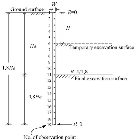
Figure 3. Representation of the Diaphragm Wall Structure
