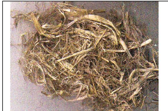
**Figure (4):** Bagasse fibers after chemical treatment
