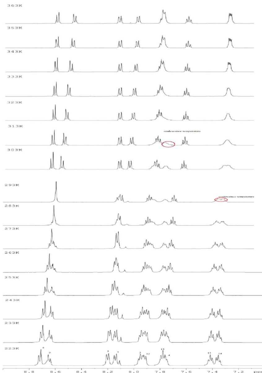
**Figure 2.** Variable-temperature  $^1\text{H-NMR}$  of benzimidazol-2-yl-quinoline
