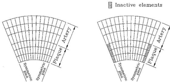
Figure 3. Transverse section of the proposed two-phase artery-plaque (TPAP) model
