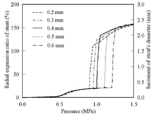
**Figure 6.** Numerical results of the TPAP model with different plaque thicknesses
