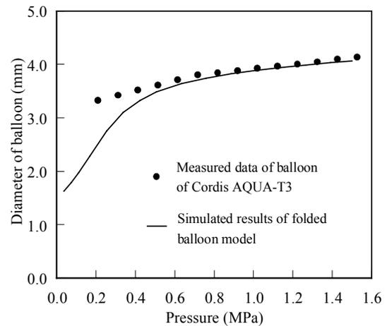
**Figure 2.** Comparison of the folded balloon model and the measured data of Cordis AQUA-T3 balloon [16]
