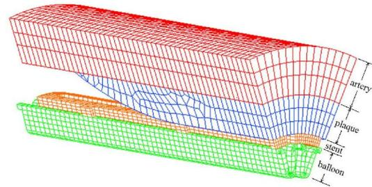
**Figure 1.** Finite element model for stent implantation
