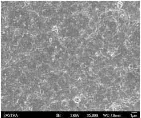
Figure 4. SEM image of nickel-tungsten (50 µm) coating
