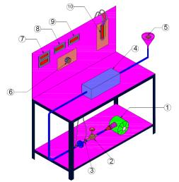
Figure 2. Schematic diagram of the experimental set up to study the convective heat transfer behaviour of the coatings [Not to scale] 1. Blower 2.Foot Valve. 3.Orifice meter. 4.Heating Section 5. Specimen. 6. Variac, 7.Temperature indicator. 8.Voltmeter. 9.Ammeter. 10.Manometer
