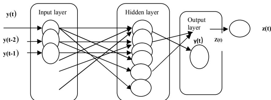
Fig 1. TDNN with two delayed inputs and one hidden layer
