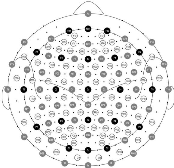
Figure 2: Electrodes designation in 10-20 system [4].
