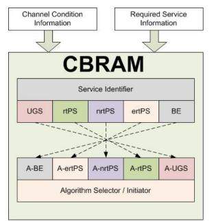
Figure 2. Proposed CBRAM Mechanism
