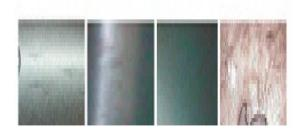
Hole, Wrinkle, Corrosion, Scrape (From Right to Left)
