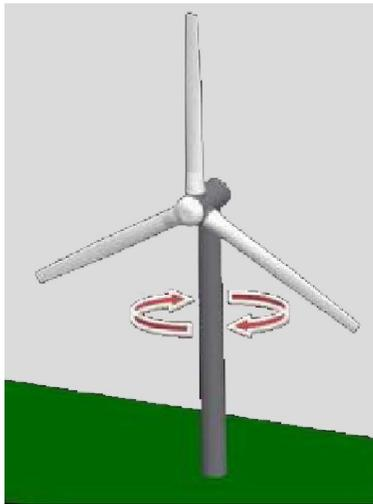
Figure 3 Turbine rotation using Yaw drive
