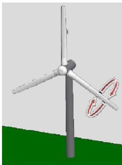
Figure 4 Pitch angle adjustment in wind turbine
