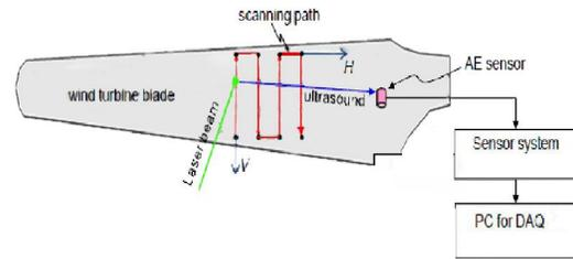
Figure 5 Wind turbine blade with AE sensor the  $b'\Omega r$  is found. The Net tangential rapidity is  $1+b'\Omega r$ . The ensuing relative velocity of the blade is  $V(B) = \sqrt{V_{in}^2 - b^2 V_{in}^2 + \Omega^2 r^2 (1+b'^2 + 2b')} \rightarrow (5)$
