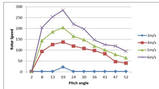
Figure 2 Rotor speed and pitch angle for various wind speed
