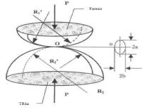
Figure 3. The biomechanic model of the elastic mesh contact of the artificial knee
