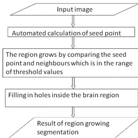
Figure 5: Step Processing of Region Growing Algorithm
