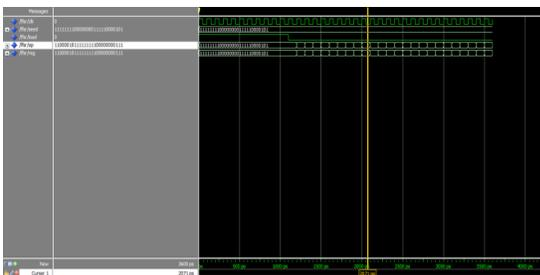
Figure 6.2 Simulation output for LFSR
