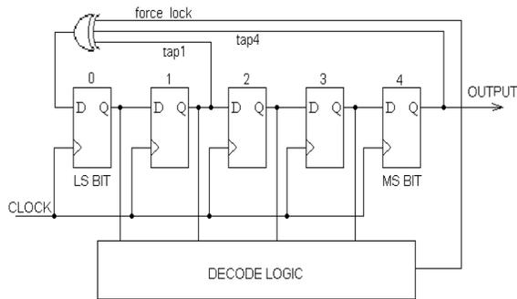
Figure 6.1 LFSR using 5 BIT
