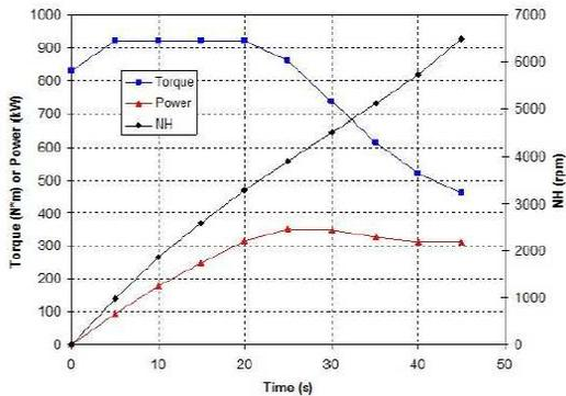
Figure 6.4 Torque, power and speed in the starting condition of the GENx-1B.
