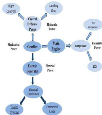
Figure 4.2 Schematic conventional aircraft power distribution system.
