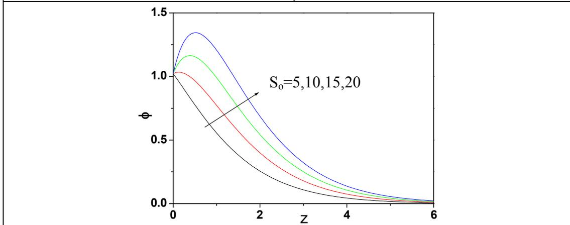
Figure 2: Effect of  $S_o$  on velocity and concentration profiles for  $\varepsilon = 0.02, t = 1, n = 0.1, \omega = 1, M^2 = 5, \eta = 1, Gr = 10, Gm = 5, R = 0.1, Pr = 0.71, Sc = 0.22, S_o = 5, m = 1.5$
