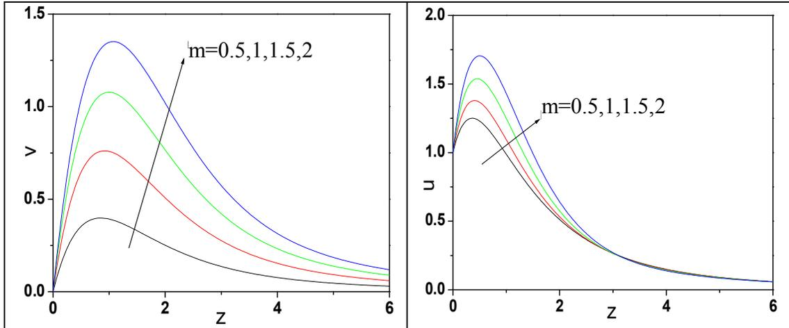
Figure 1: Effect of  $m$  on velocity profiles for  $\varepsilon = 0.02, t = 1, n = 0.1, \omega = 1, M^2 = 5, \eta = 1, Gr = 10, Gm = 5, R = 0.1, Pr = 0.71, Sc = 0.22, S_o = 5, \delta = 5$
