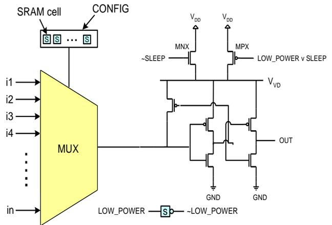
**Figure 6. Basic switch design**
