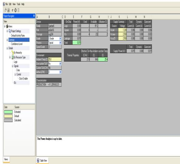
**Figure 11. Power result of FPGA in SPARTAN 6**
