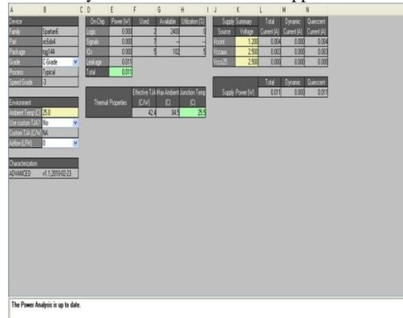
Figure 17 . Power result of FPGA in SPARTAN 6
