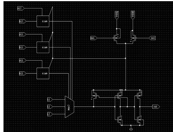
**Figure 2. Schematic diagram of the existing routing switch**
