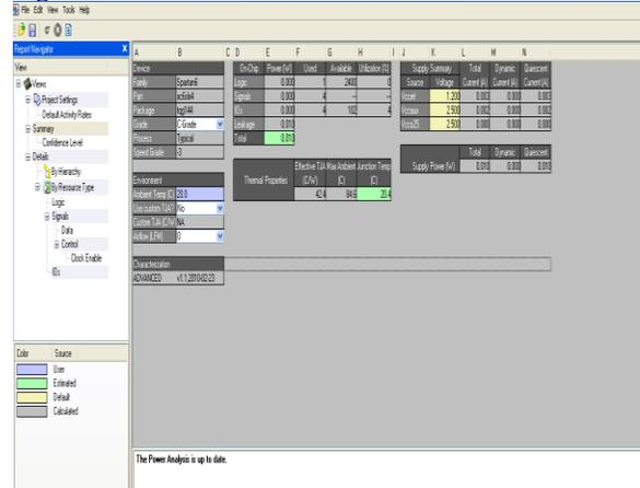
**Figure 14. Power result of SRAM in SPARTAN 6**
