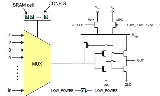
**Figure 5. Basic switch design**
