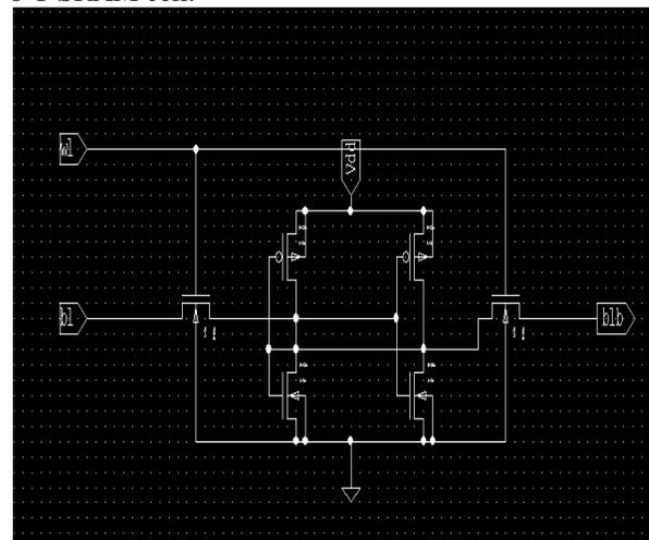
**Figure 1. Schematic diagram of 6-T SRAM cell**
