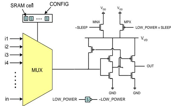
**Figure 4. Basic switch design**
