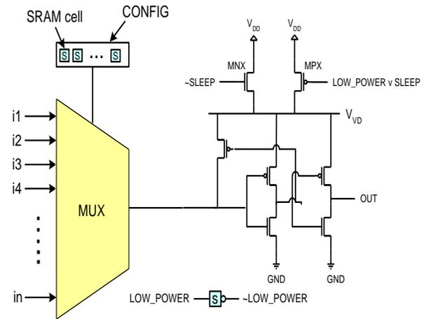
**Figure 3. Basic switch design**
