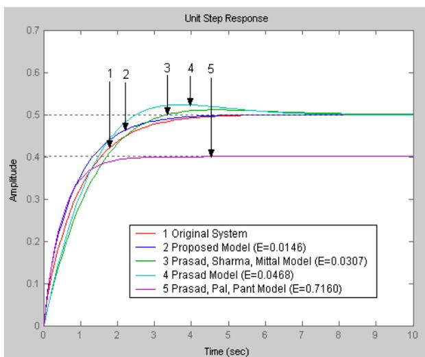
Figure 4: Unit step response curves for  $G_{21}(s)$
