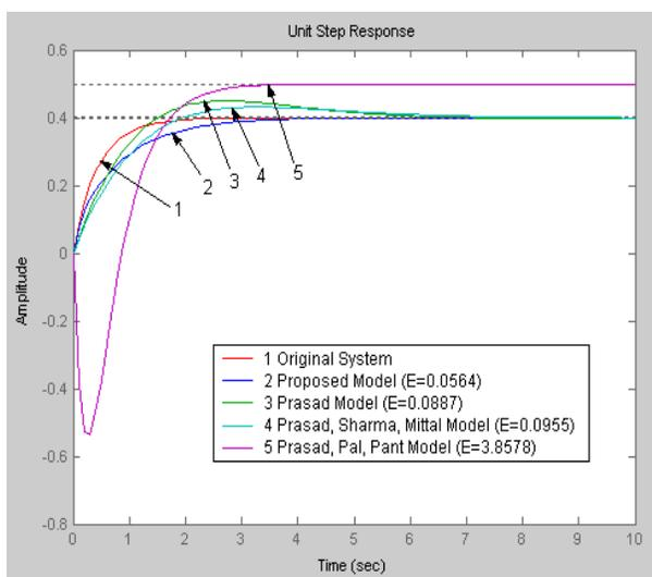
Figure 3: Unit step response curves for  $G_{12}(s)$
