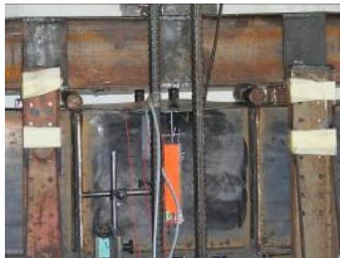
**Figure (6):** local buckling for slender flange specimens during loading course and after failure
