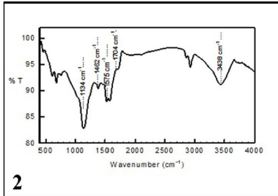
**Figure 2:** Fourier transform infrared spectra of MWCNTs synthesized at 600 °C and then oxidized in concentrated acid for 6 hrs.
