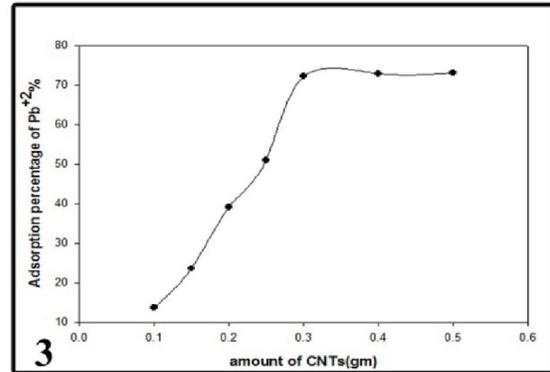
**Figure 3:** Shows the effect of the MWCNTs on the adsorption of Pb<sup>2+</sup>.
