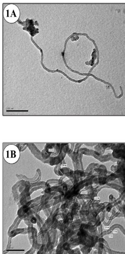
**Figure 1 (A, B):** Transmission Electron Microscopic (TEM) photos of MWCNTs synthesized at 600 °C and oxidized in concentrated acid for 6 hrs.
