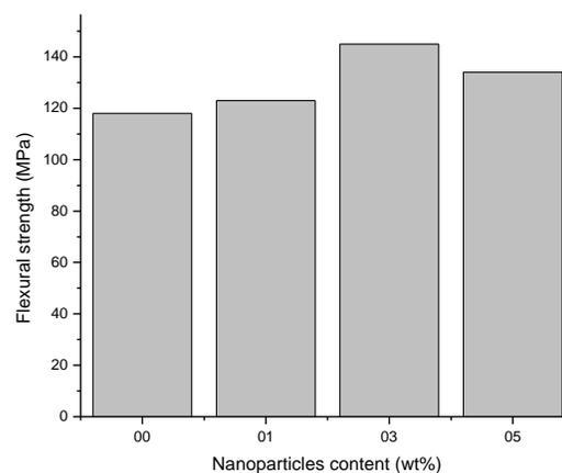
Figure 3. Plot of flexural strength for composites
