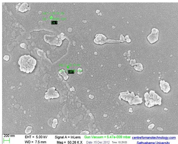
Figure 8. SEM image of glass fibre with 5 wt% of nanoparticles
