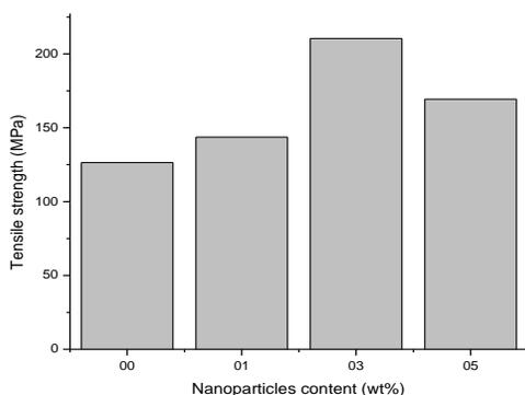
Figure 1. Plot of tensile strength for composites
