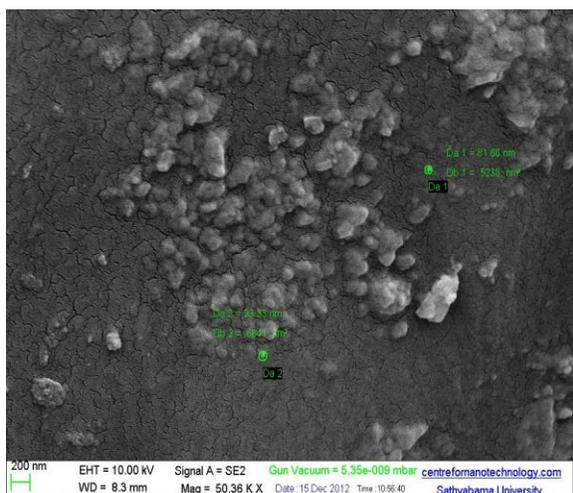
Figure 7. SEM image of glass fibre with 3 wt % nanoparticles
