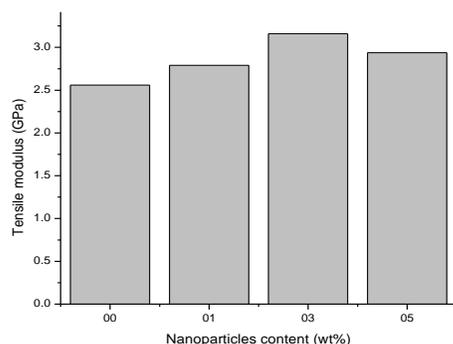
Figure 2. Plot of tensile modulus for composites
