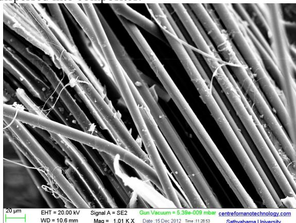
Figure 5. SEM image of glass fibre with 0 wt % nanoparticles
