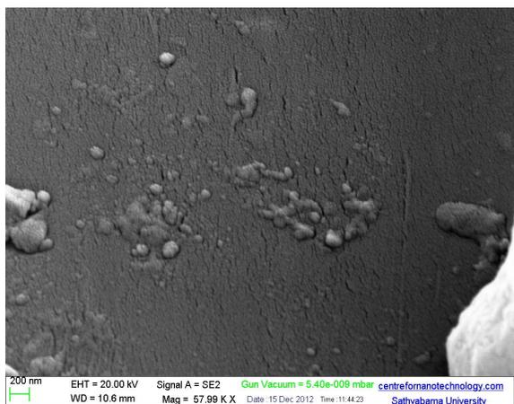
Figure 6. SEM image of glass fibre with 1 wt % nanoparticles
