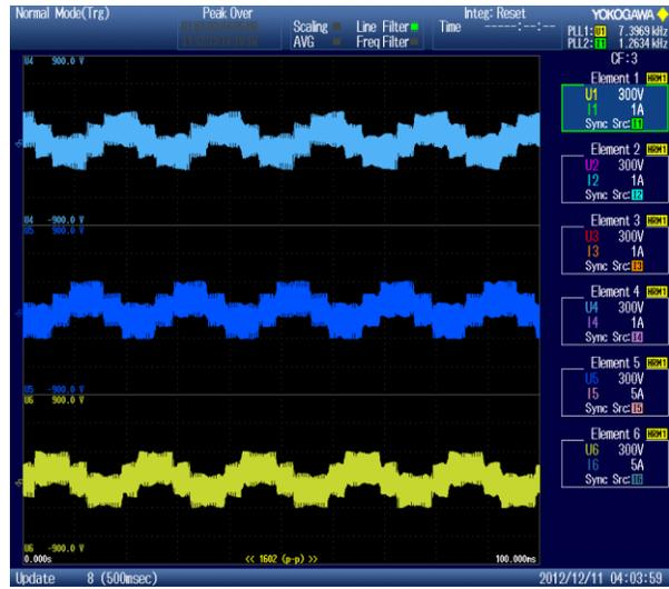
Figure 9. SPWM; M.I.=0.8; Line to Neutral Voltage
