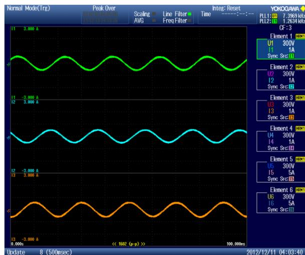
Figure 10. SPWM; M.I. =0.8; Line to Line Current
