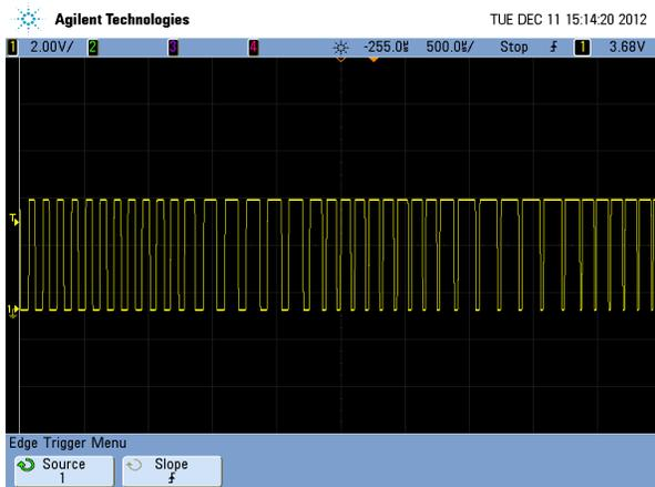
Figure 7. DSO Output of RFPWM
