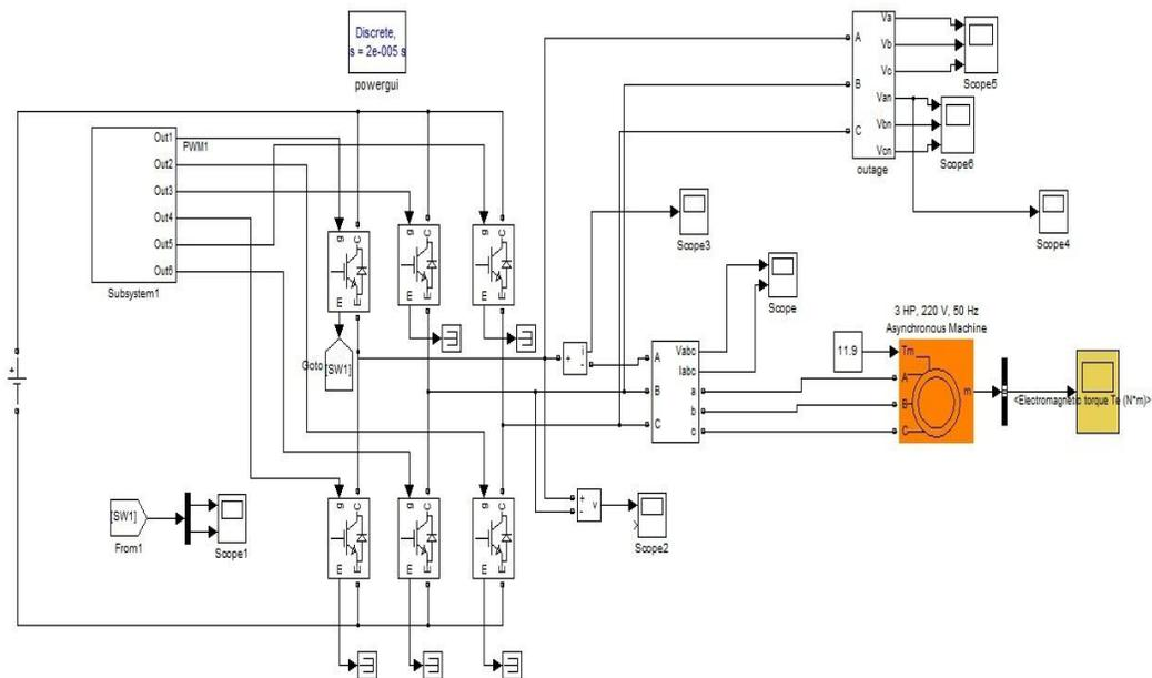
Figure 2. Matlab Simulation model of the Inverter circuit
