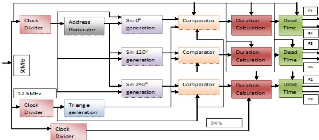
Figure 1.FPGA implementation of the proposed scheme
