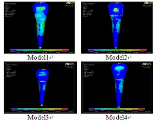
Figure 5. Von Mises distribution on dentin lingual surface in different models
