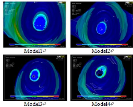
Figure 6. Von Mises distribution on apex of root in different models
